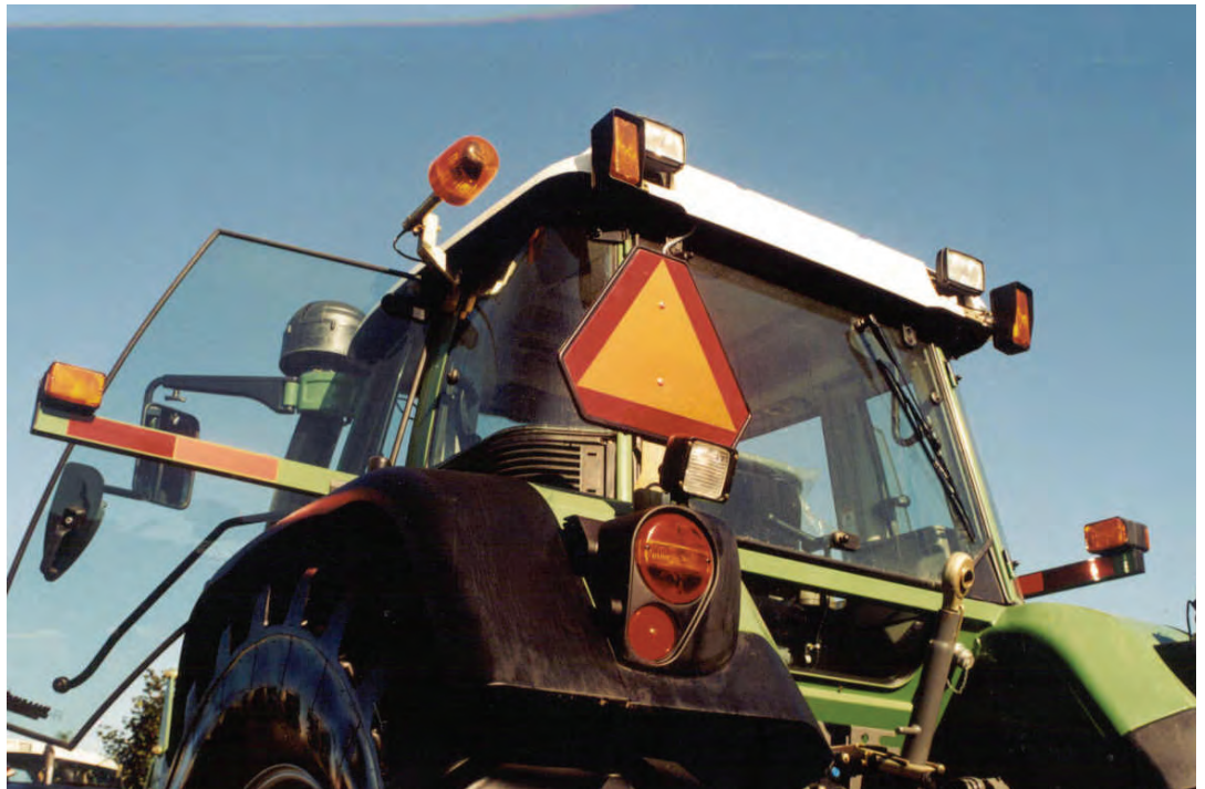
Machinery travelling slower than 40 km/h must have a slow moving vehicle sign attached to the back of the self-propelled farm equipment and any towed implement.
